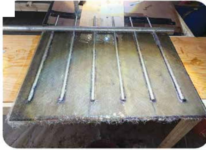
January 29: Laying up the rudder
